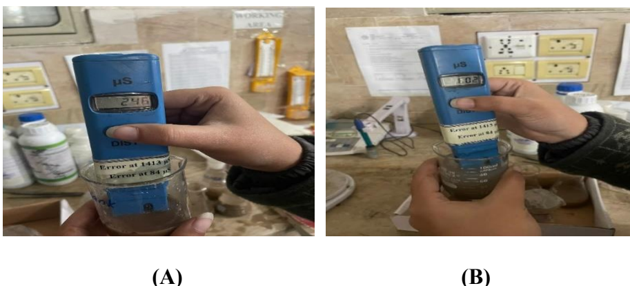
Figure 3.5 Determination of Electrical conductance of soil and Biochar
