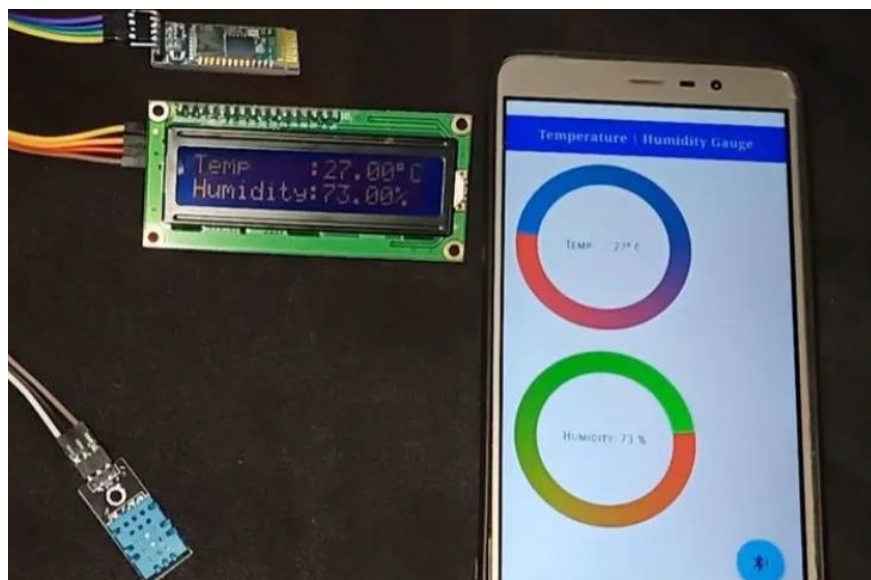
Figure 4-13: Mobile application for end-user environmental monitoring
