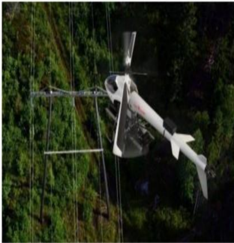
Figure 2.3: Transmission lines helicopter-based inspection [6]
