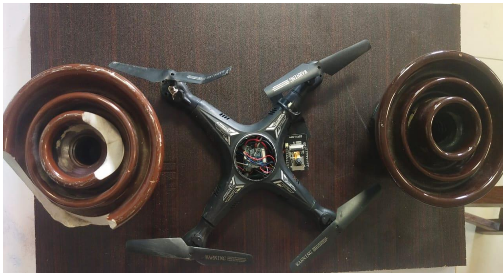
Fig 4.1 Healthy and unhealthy insulator and drone
