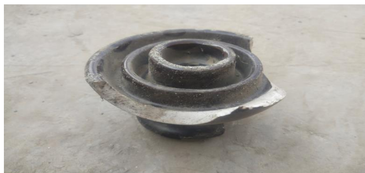
Figure 3.8: Unhealthy insulator result
