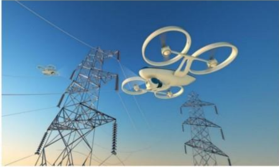
Figure 2.6: Transmission lines inspection through UAV [14]
