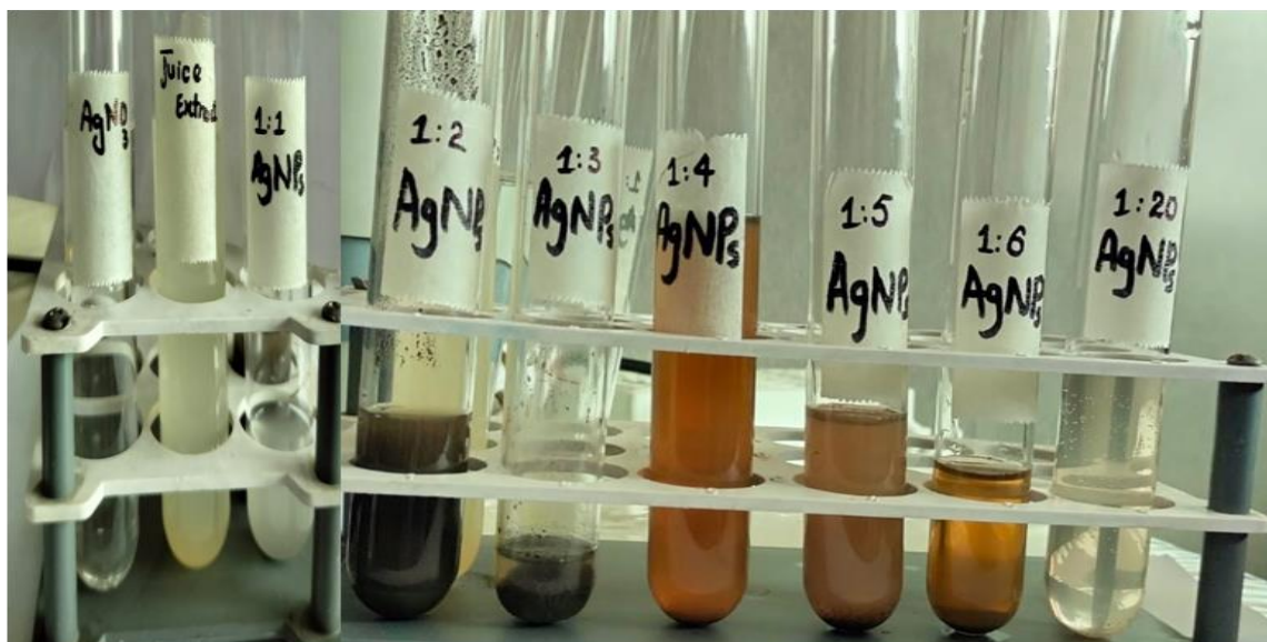
Figure 4. 8: Indication of colour change in different ratios v/v (JE/SNS): The reddish-brown colour is visible in 1:4 ratio.
