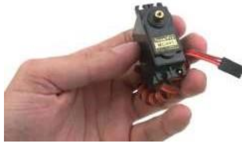
Figure 3.6.3: MG-995 Servo motor[13]
