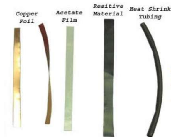
Figure 3.5.2a : Flex sensors materials-1[9].
