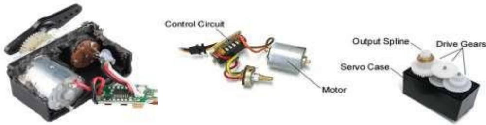
Figure 3.6.2-a: Inside structure of a typical servo motor-part-1[12].
