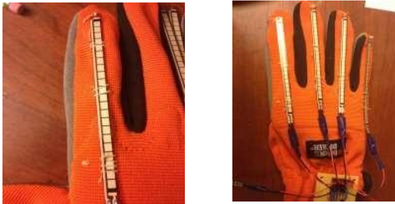
Figure 4.10 Attaching flex sensors on glove
