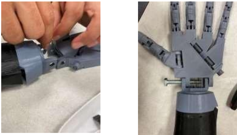
Figure 4.8 Attaching Hand and Wrist together
