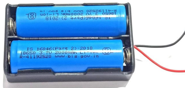
Figure 4.7: The Battery Pack (3.7V Li-ion Cells)
