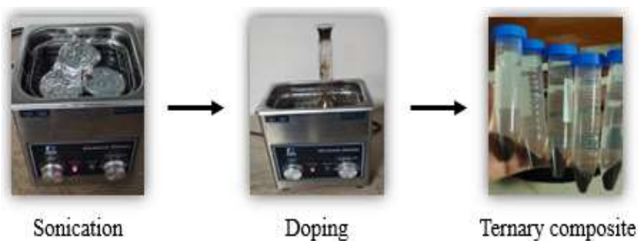
Figure 3.5 Synthesis of copper oxide doped copper ferrite doped graphene oxide (CuO/CF/GO) ternary composite.
