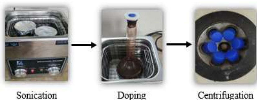
Figure 3.4 Synthesis of copper oxide doped copper ferrite (CuO/CF) binary composite.
