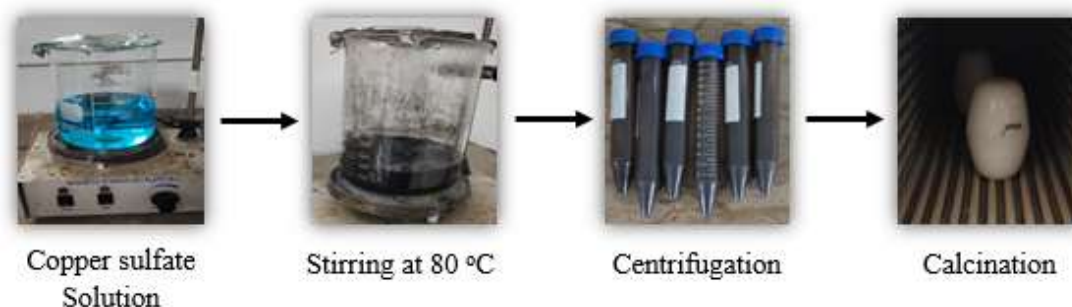
Figure 3.3 Synthesis of copper oxide ( \text{CuO} ) nanoparticles.
