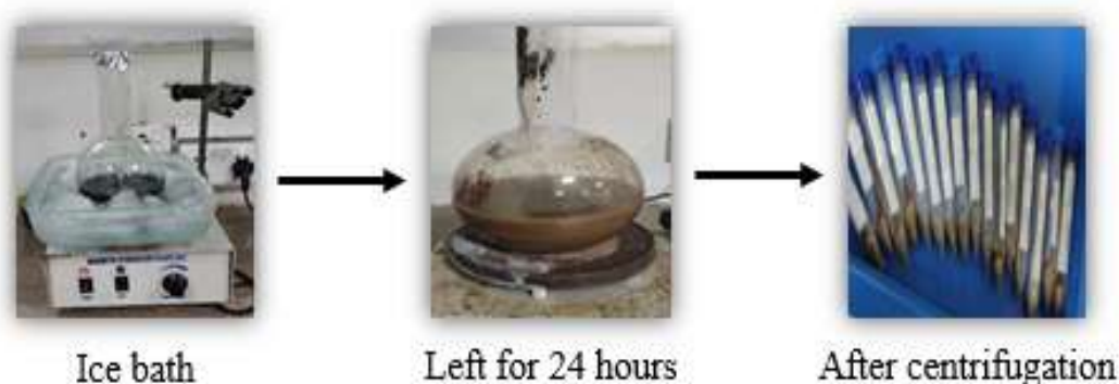
Figure 3.1 Synthesis of graphene oxide (GO).
