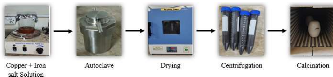
Figure 3.2 Synthesis of copper ferrite ( \text{CuFe}_2\text{O}_4 ) nanoparticles.
