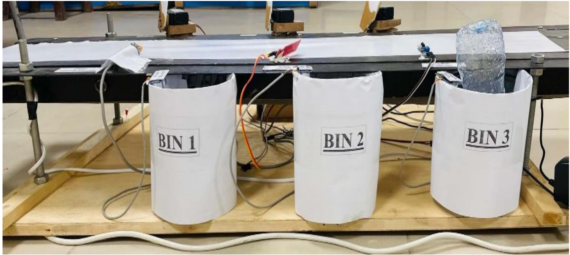
Figure 4. 30: Waste Collection Bins Equipped with Ultrasonic Sensor
