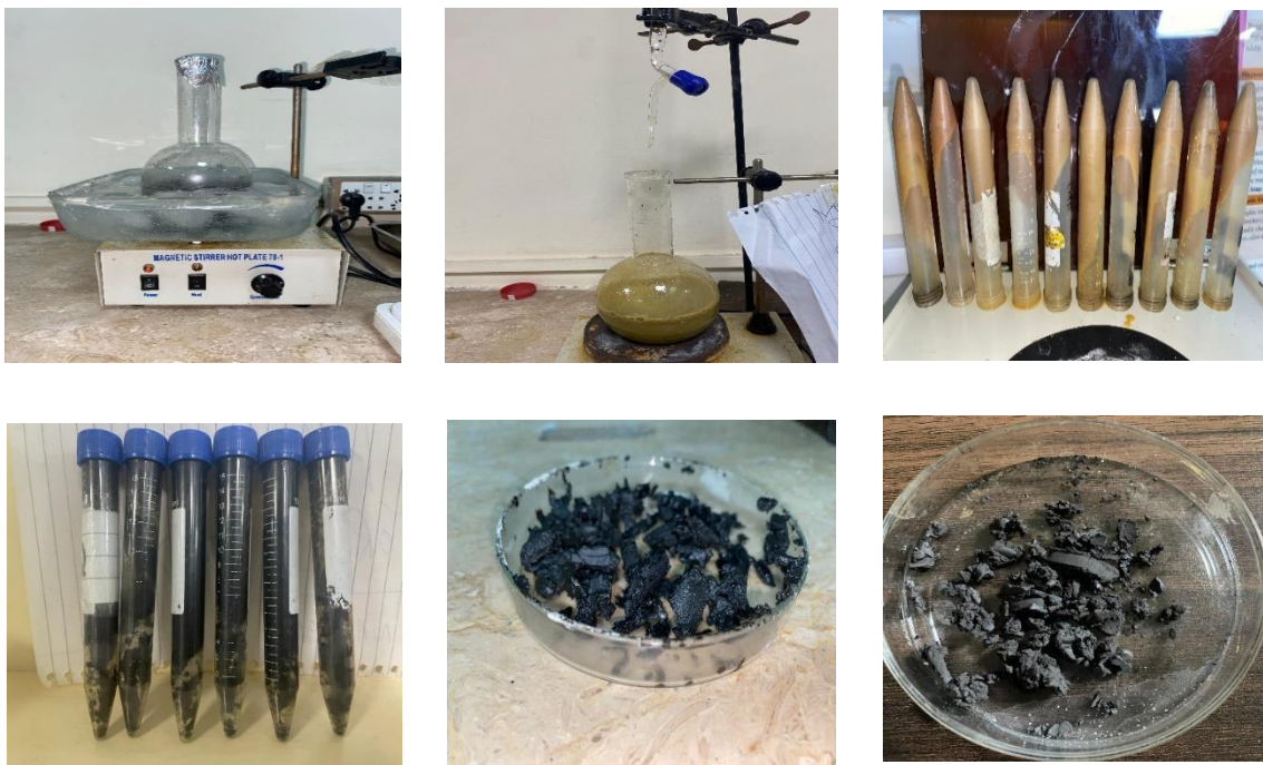
Figure 3.1 a) Reaction start b) Reaction Stop c) Centrifugation d) Partially Dried GO in falcon tubes e) Partially dried GO in petri dish f) Dried GO in petri dish
