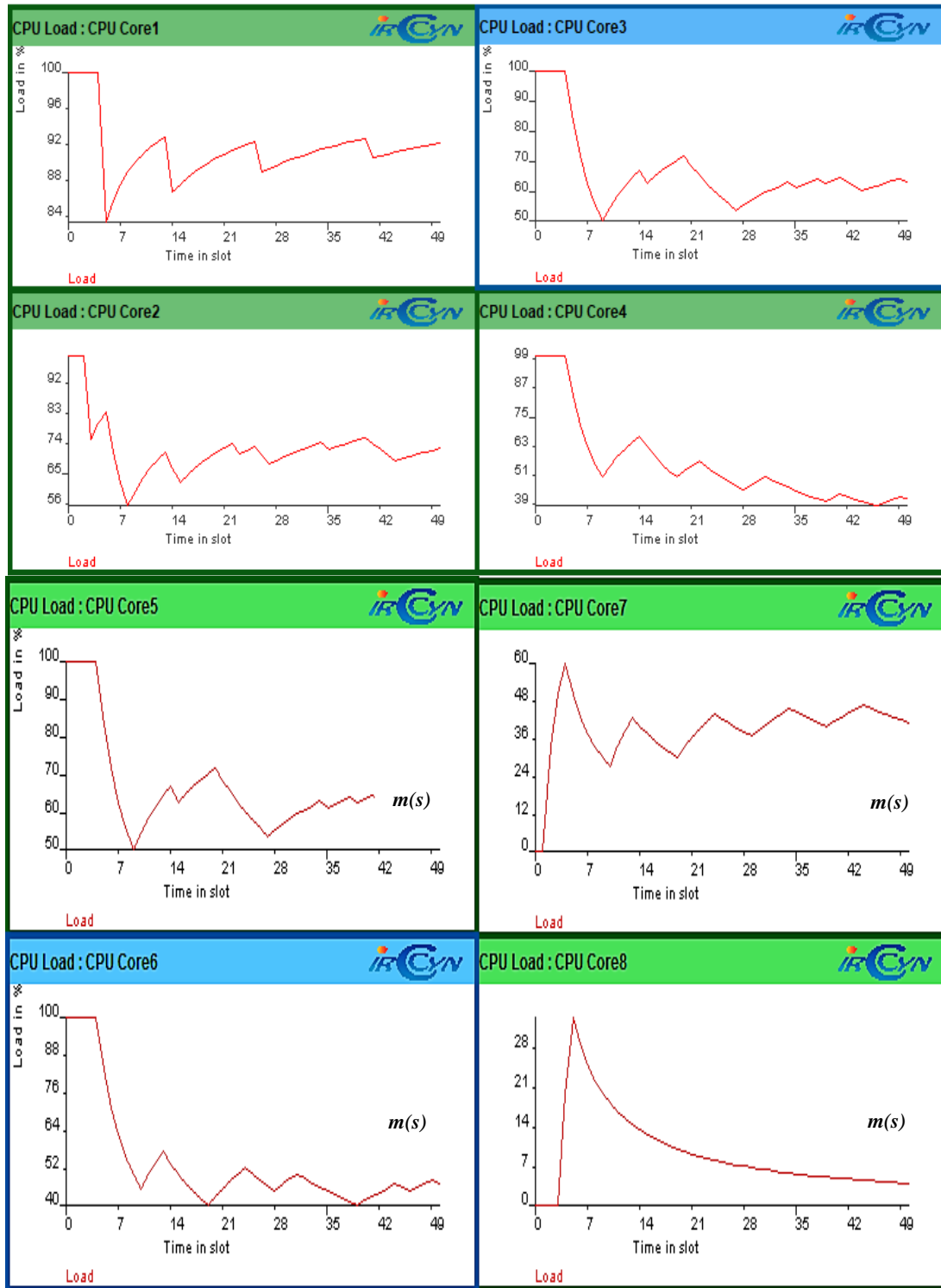
Figure 5.43 CPU load on the core p_1, p_2, \dots, p_8 under u_i > 62.5\% at 624 MHz.
