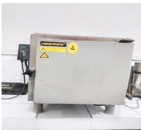
Figure 3.1 Muffle Furnace for the synthesis of Biochar
