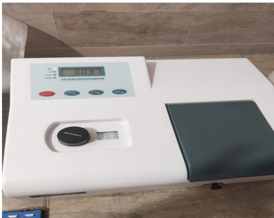
Figure 3.7 UV Spectrophotometer for analyzing phosphorus content
