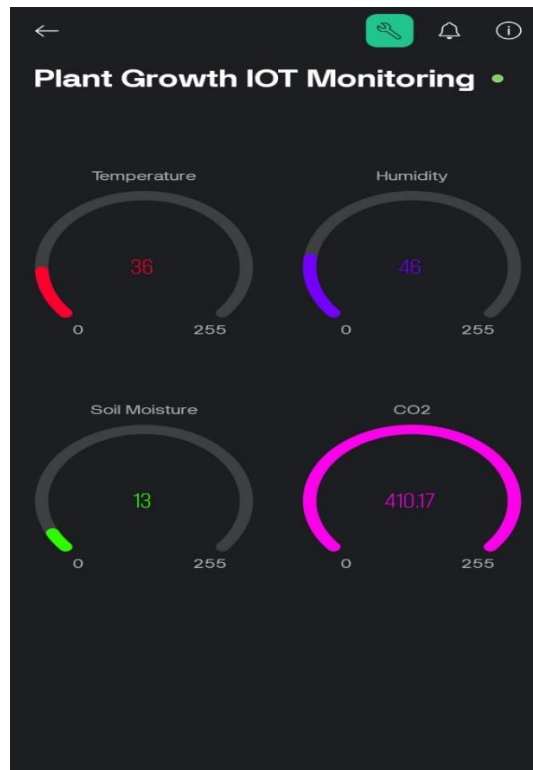
Figure 16 Parameters Output on Blynk Application via ESP8266
