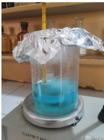
Fig 3.2. Solution of Lanthanum hex nitrate, Strontium nitrate, Copper nitrate and Titanium oxide heat and stir about 120^{\circ}\text{C}
