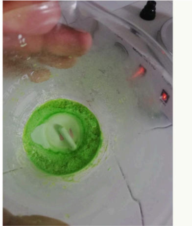
Fig.3.1. Gel obtained at 80C 0 continuous heating and stirring 4 hours
