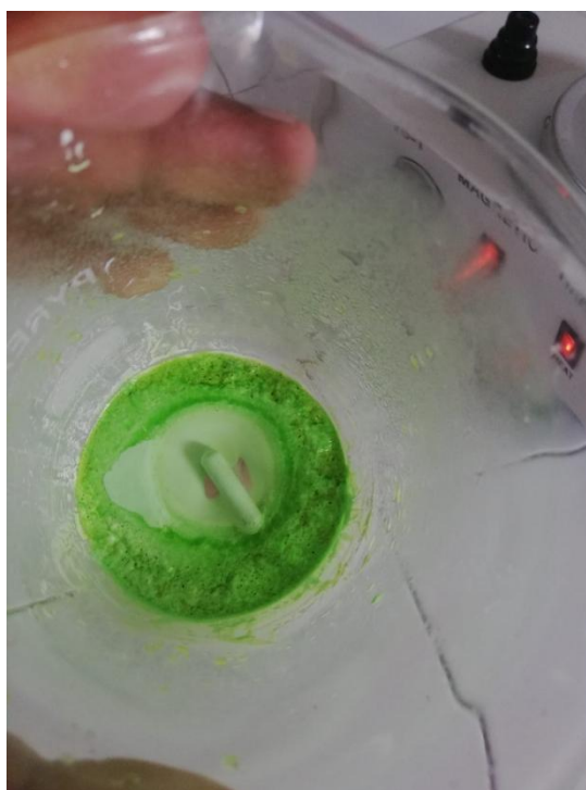
Fig.3.1. Gel obtained at 80C 0 continuous Heating and stirring 4 hours
