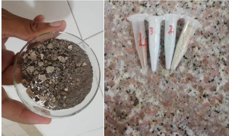
Fig 3.3: Powder form sample obtained after dry and Sintering at 900 0 C
