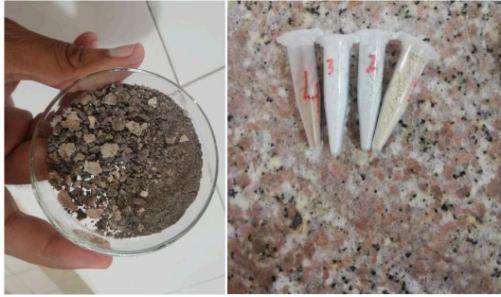
Fig 3.3: Powder form sample obtained after dry and sintering at 900°C
