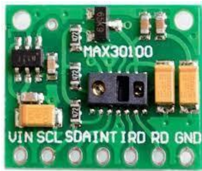
Fig2.2.25 (v) Pulse Oximeter (Module Max30100
