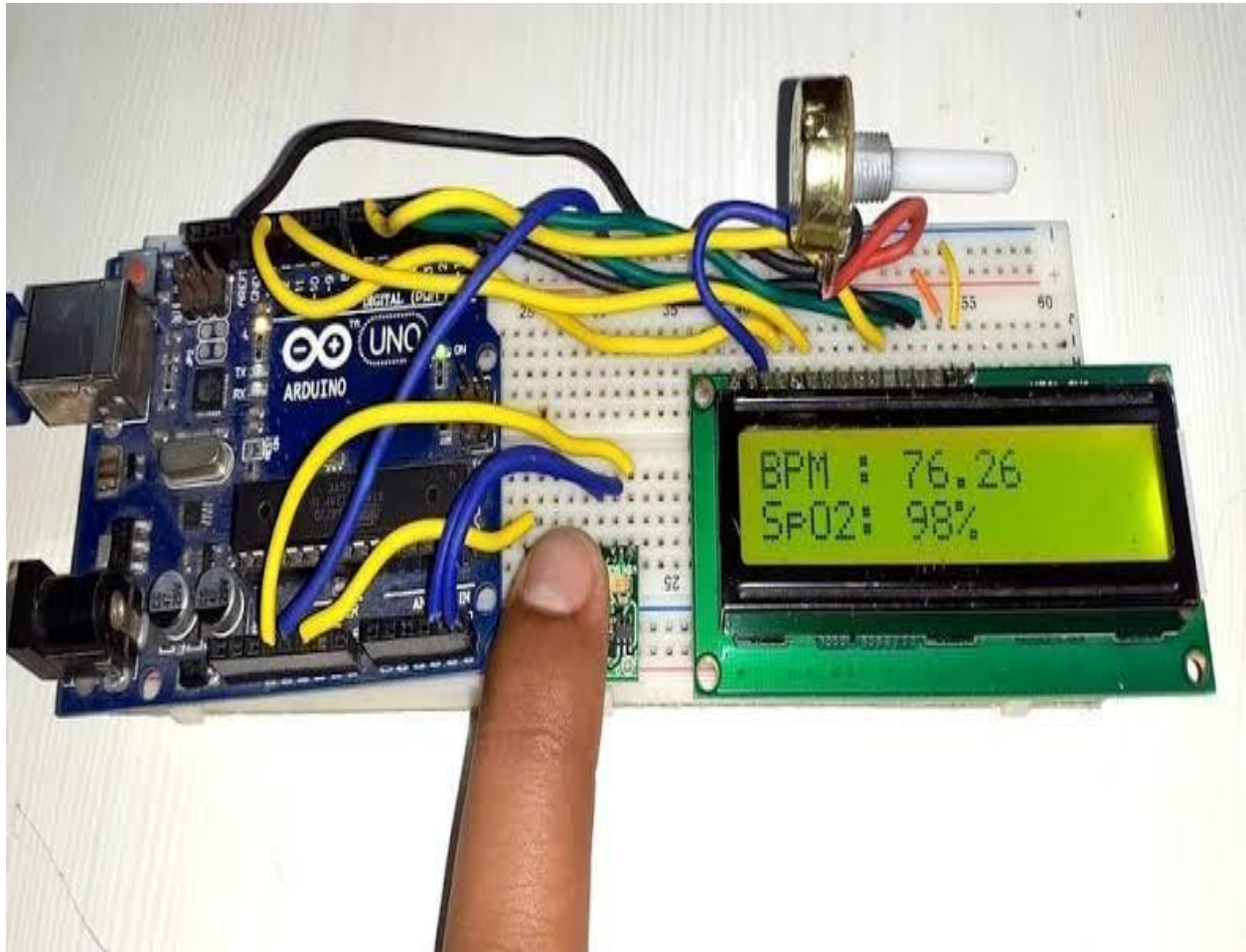
Figure 7.6 Sensor used for measuring pulse oxy
