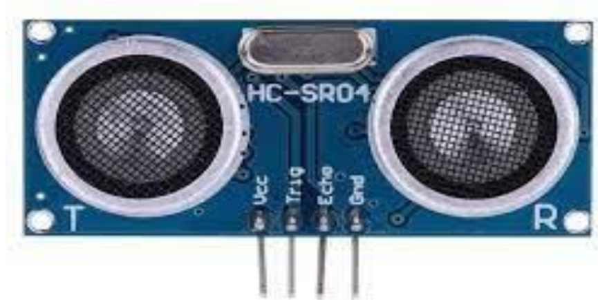
Fig2.2.5 (vi) Sonar Sensor (HC-SR04 ultrasonic sonar)
