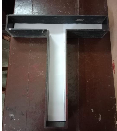
Figure 3.5.5: Stride Length Test Apparatus
